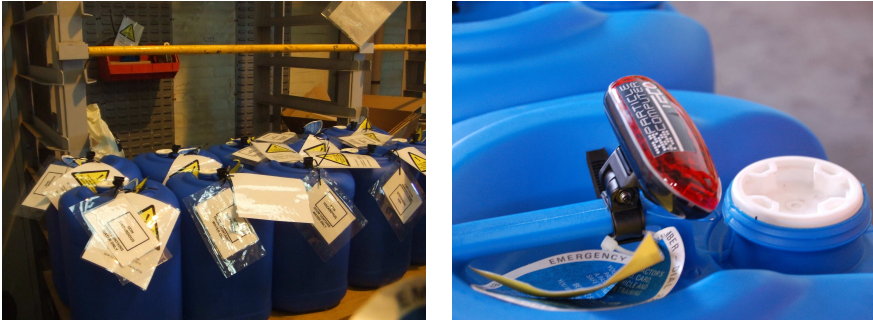
Figure 3.1: Application trial in Hull, UK: Chemical containers stored in a warehouse (left); Detail with a sensor node attached to a container (right).
