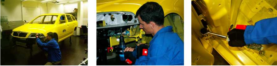
Figure 6.1: A car assembly worker performing several activities. Sensors are both worn by the worker and attached to the tools and car parts.
